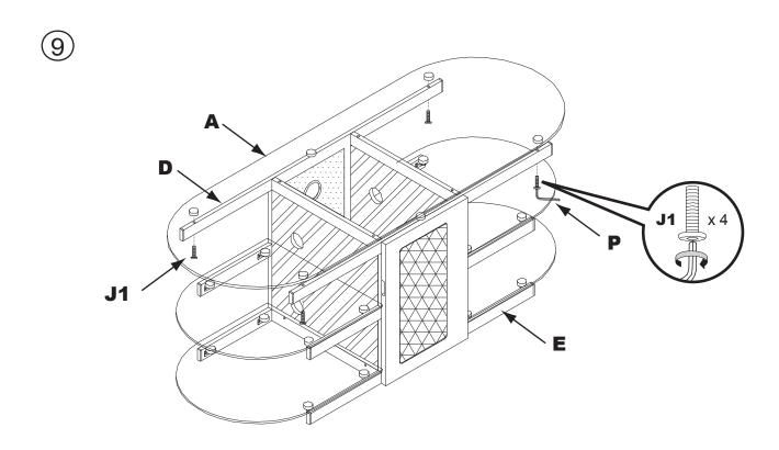
9- Turn unit to upright position,fasten top glass (A) to the frames (D&E) with screws (J1).
